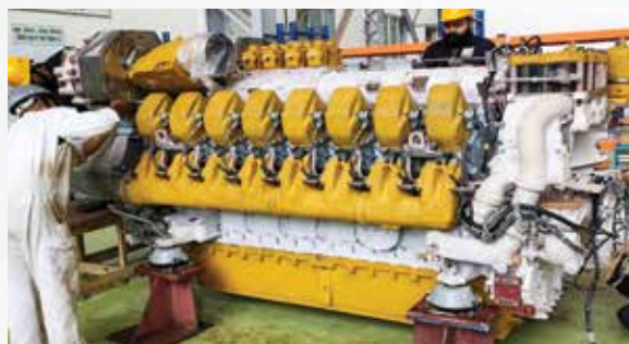
Assembly of Engine Post W6 Routines/ Major Overhaul
